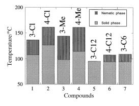
Fig. 2 Comparison of the nematic range (°C) for the different compounds
