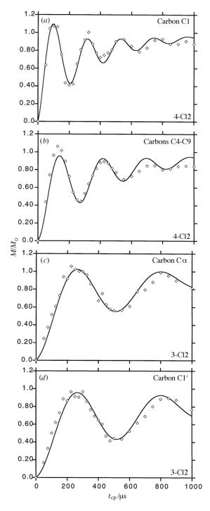
Fig. 5 Intensity variation of some resonances as a function of the contact time during the cross-polarization experiment. For **4-C12** at  $80.1\,^{\circ}\text{C}$ : (a) carbon C1, (b) aliphatic center peak containing 6 carbons For **3-C12** at  $84.1\,^{\circ}\text{C}$ : (c) carbon  $C\alpha$ , (d) carbon C1'
