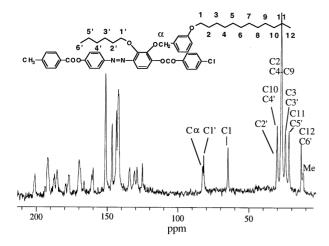
Fig. 1 Proton-decoupled  $^{13}\mathrm{C}$  spectrum of 3-C12 in the nematic phase at 67.942 MHz with aliphatic carbon labelling. Acquisition parameters: cross-polarization (CP) with flip-back, contact time = 1 ms, recycle delay = 6 s, number of scans = 300, temperature = 84 °C
